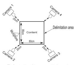
Fig. 3 Position of the cameras with Content 2.
